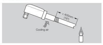
It can be fitted using a ½" viewing tube that should be aligned on the first flame third, as this is where the highest UV radiation is generally found. The inside of the steel tube should not be coated and the tube should be directed at the flame from above so that no dirt collects in front of the UV sensor.
